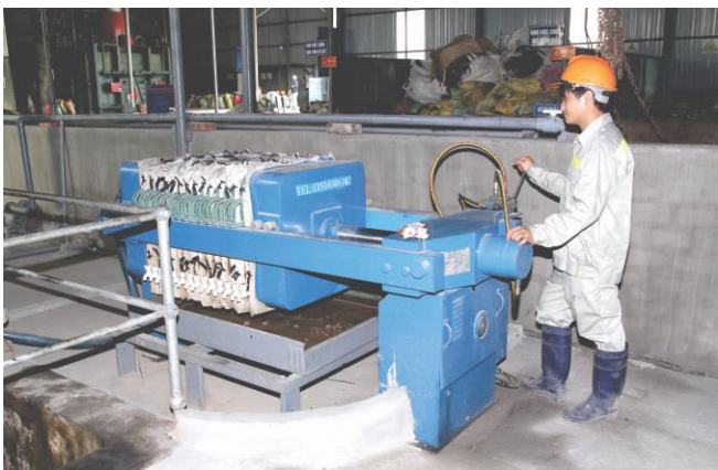
Processing system for oil-contained sludge
